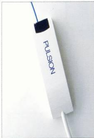
Probe connected to the optical module of the CeVOX – in vitro calibration
