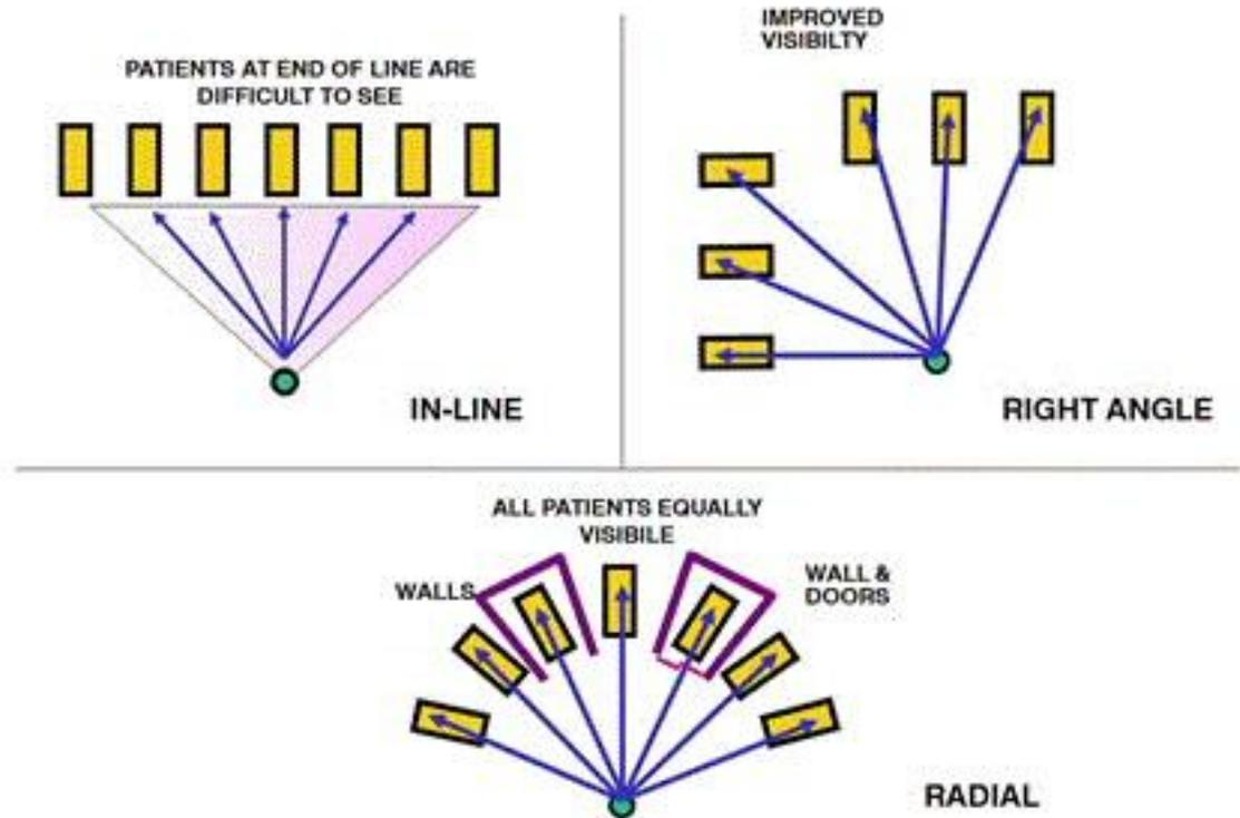
**Figure 1: Linear layouts restrict visibility. Creating a right angle can improve on this, but can create awkward spaces. a radial layout allows all rooms to be visualized, and all staff to be proximal with no wasted space.**
