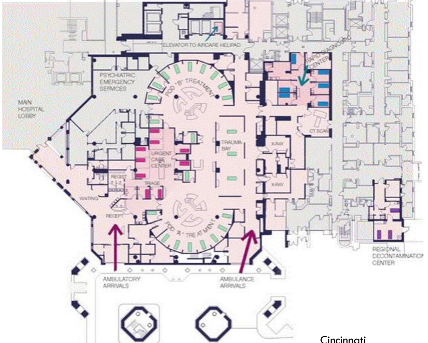
Figure 4: Radial layout concept introduced at University Hospital.
